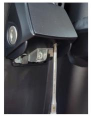
2.1 Unscrew the upper battery mount from the plate.
