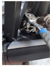
2.2 Unscrew the original battery mounting plate with hinge suspension.
