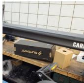
4.1 Mount the Adapter with the Model X and the Bosch battery mount on it to the frame. Use the supplied M8 bolts on the top. The original nuts and bolts can be used on the underside (up-side-down).
