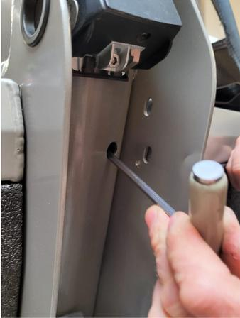
**1.1** Remove the battery from the bicycle and slightly loosen the 2 Allen screws under the battery (maximum 3 rotations). **ATTENTION: never unscrew these bolts completely!**
