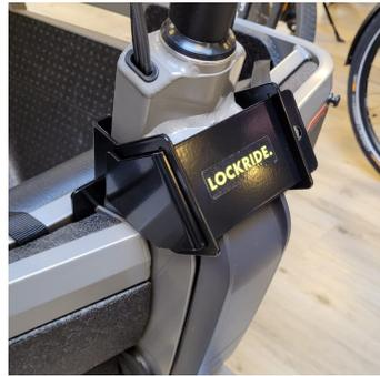
3.3 Mount the slide in the bracket and attach the Abus Diskus lock.
