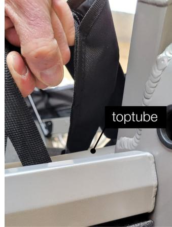
**1.2** Lift the top tube as far as possible to create space between the foam and the top tube.
