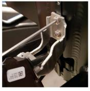
2.4 Dismount the bracket from the frame using the Inbus tool.
