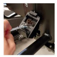
2.1 Unscrew the two housing parts with a Torx screwdriver.
