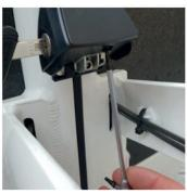
1.2 Unscrew the lock cap at the bottom with a Torx screwdriver.
