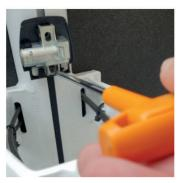
**1.4** Unscrew the two Inbus screws.
